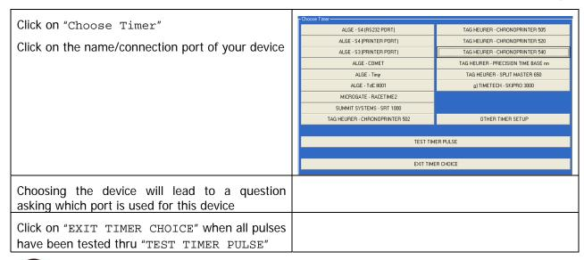
It is important to test the timer using the TEST TIMER IMPULSE button and test ALL impulses: Start, Speed, Intervals and Finish. This will also helps finding which Channel each impulse is connected to (this information is used to configure the timer (F3)
